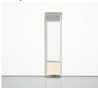
Fig. 7-1: A standard cuvette showing the ideal sample volume.
