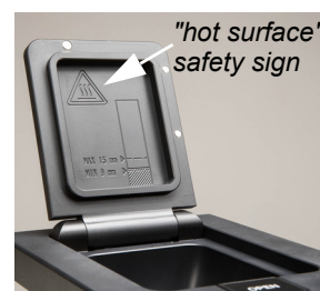
Fig. 2-7: "Hot surface" safety sign on the inside surface of the cuvette module lid (left) and on top of the thermal insulation cover (right)
