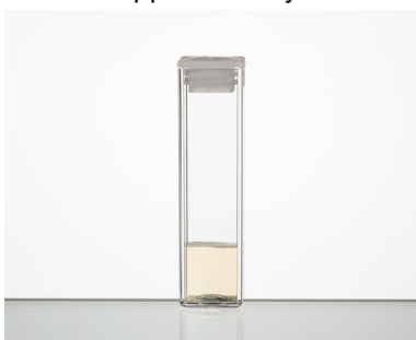
Fig. 9-1: A standard cuvette showing the ideal sample volume.
