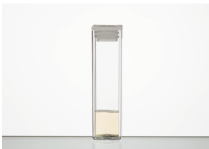
Fig. 10-1: A standard cuvette showing the ideal sample volume.
