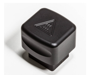
Fig. 2-7: "Hot surface" safety sign on the inside surface of the cuvette module lid (left) and on top of the thermal insulation cover (right)
