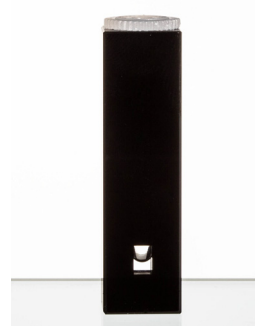
Fig. 7-2: Small-volume cell showing the minimum sample volume (20 \mu\text{L} )
