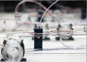
FAB FOUR: This is a close-up shot of the SEAL AutoAnalyzer. In the tubes, the bubbles separate samples. The instrument can run up to four different analyses at once on one sample; it measures how much phosphate, silica, nitrate and ammonia are in the water.
