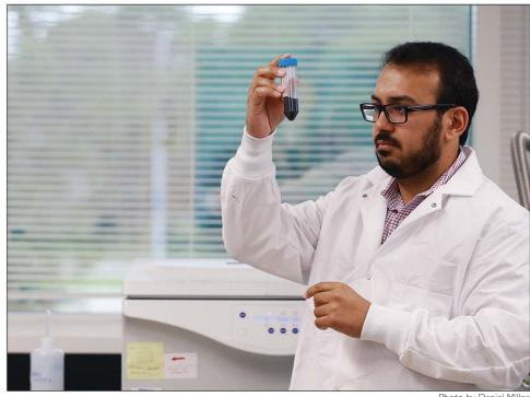
IN THE LAB: Dr. Reza Rizvi, assistant professor of mechanical, industrial and manufacturing engineering, looked at a dispersion of graphene that was produced using his rapid and scalable exfoliation process. This new process can enable low-cost, flexible and printable electronic devices.
